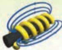
The magnetic field can be made even stronger by placing an iron bar in the center of the coil. This has a big effect on the electromagnetic power.
