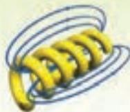
By coiling the wire into a coil and concentrating the magnetic field it produces a stronger field. When electrical current produces a stronger magnetic field.
