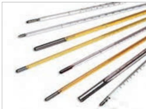
Fig. 26: Laboratory liquid - expansion thermometer
