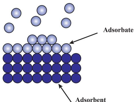
Fig.5: Adsorption process
