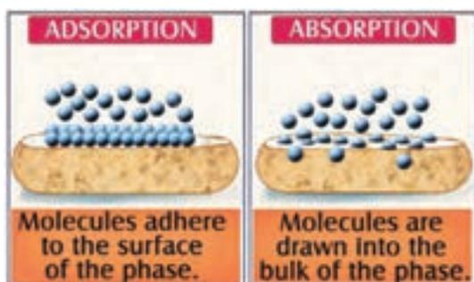
Fig 6: Adsorption and absorption
