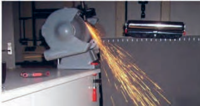
Figure 2: Spark test of a high carbon steel
