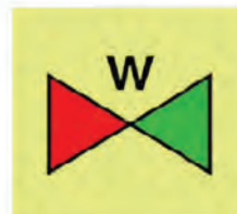
Fire main section valve
