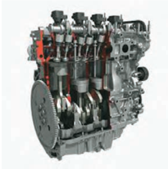
Fig 24: A four-Stroke Engine
