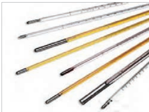
Fig. 26: Laboratory liquid - expansion thermometer
