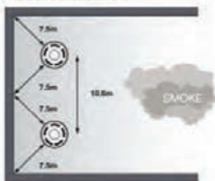
Heat detector spacing (under flat horizontal ceiling)
