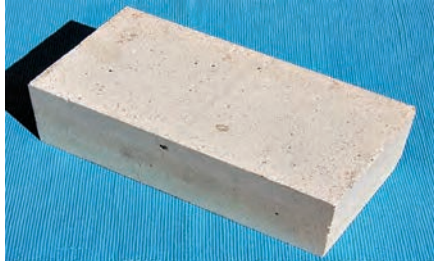
a heavy and dense refractory brick
