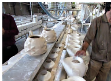
An example of a ceramic pottery made by slip casting
