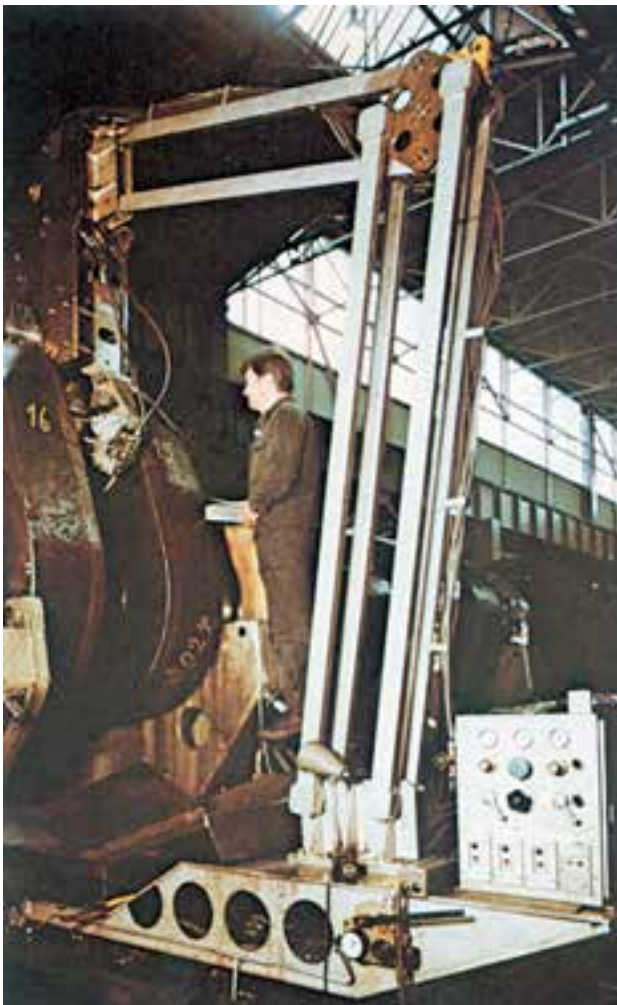
□ Machine finishing of a crank pin
