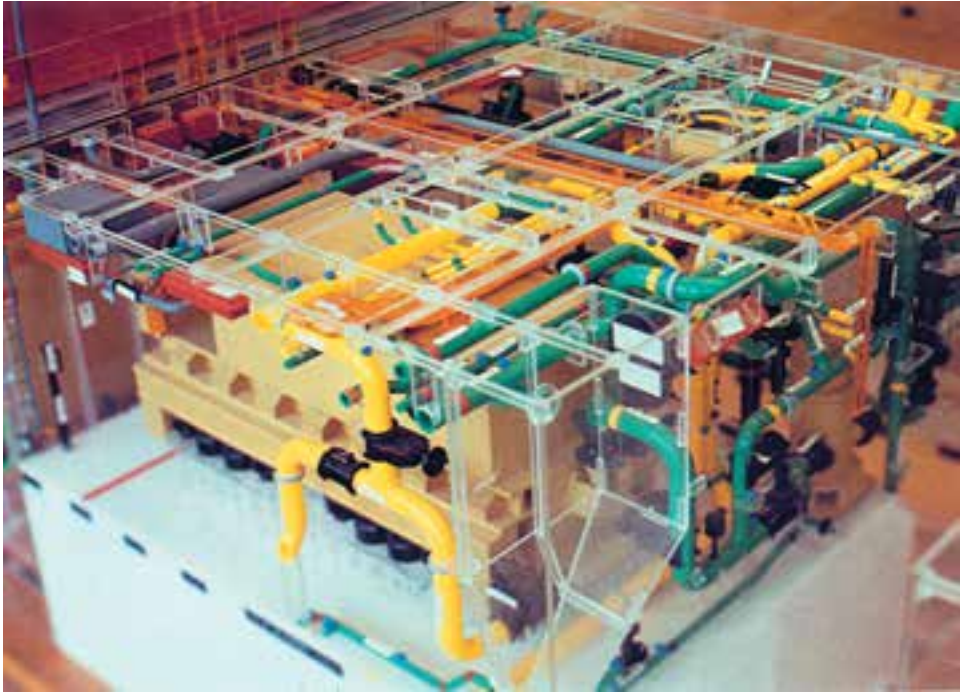
Part of auxiliary engine room model
