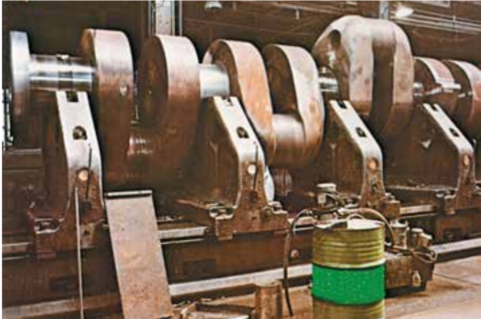
□ Crank shaft on the turning lathe
